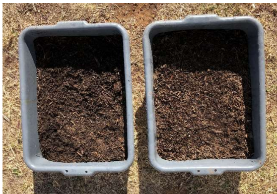
Preconditioned soil beds ( 12 \pm 2\% moisture)
