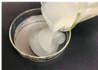
Guar gum solution cast in Petri dishes
